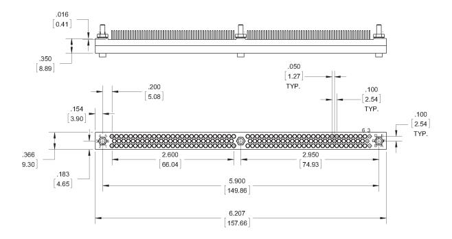
ONLY AVAILABLE WITH HARDWARE STYLE POLARIZED GUIDES WITH MOUNTING STUD (B)
